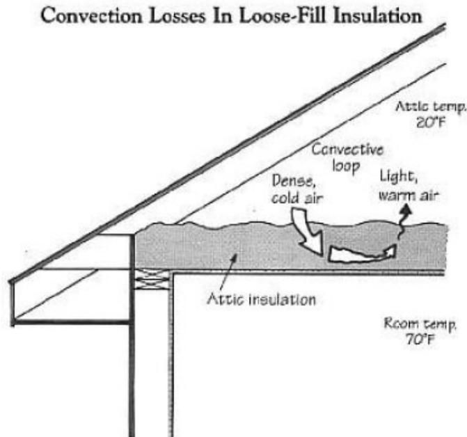
*At very cold temperatures, when the temperature difference across the attic insulation reaches a certain critical point, convection within the insulation can reduce R-value.*
