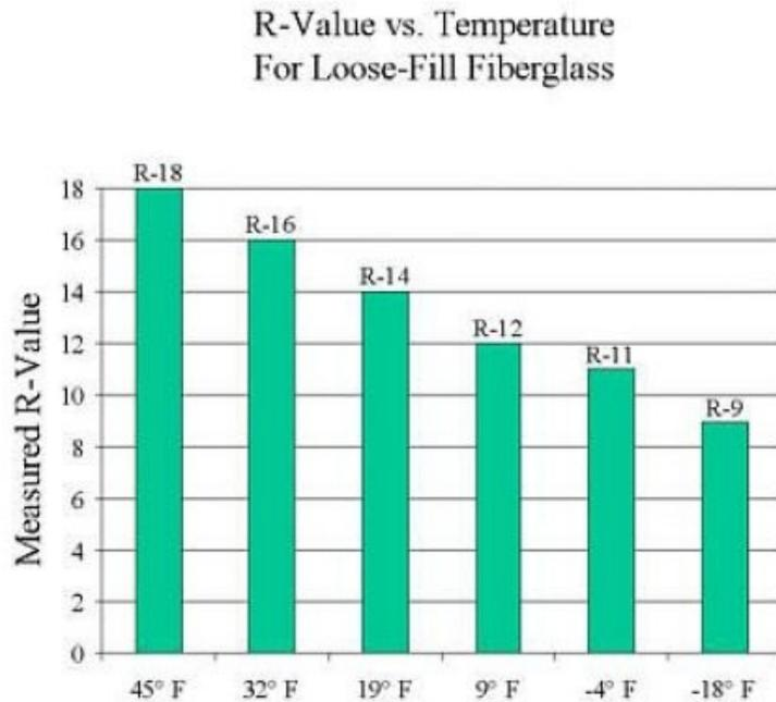
*In full-scale attic tests at Oak Ridge national Laboratory, the R-value of 6 inches of cubed loose-fill attic insulation progressively fell as the attic air temperature dropped. At -18 F, the R-value measured only R-9. The problem seems to occur with any low-density, loose-fill fibrous insulation.*
